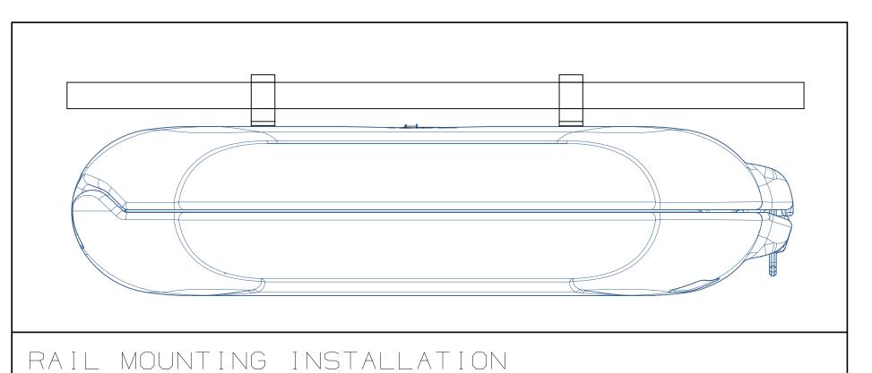
WHEN RAIL MOUNTING THE HOUSING HORIZONTALLY, IT MUST BE DONE IN THE ORIENTATION SHOWN ABOVE. THIS WILL ENSURE CORRECT FUNCTION OF THE PRODUCT.
